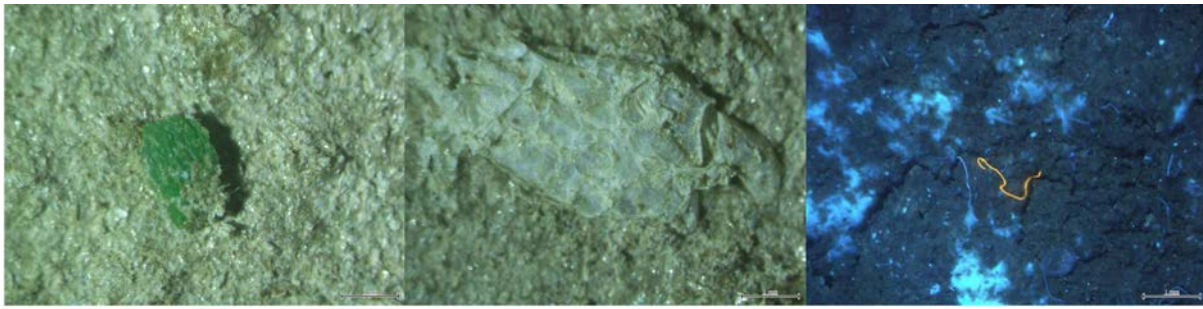
Figure 4: Example of microplastic sampled in Sugashima, Mie. From left to right: plastic particle, plastic film and different polymer types of microfibers under UV light.
