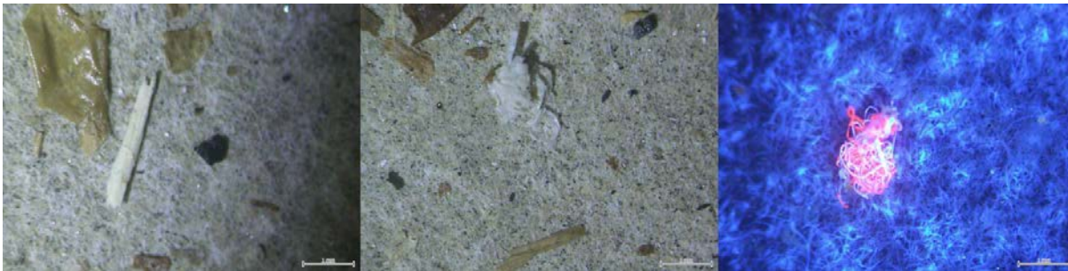
Figure 5: Example of microplastic sampled in Sugashima, Mie. From left to right: plastic particles, plastic film and different polymer types of microfibers under UV light.
